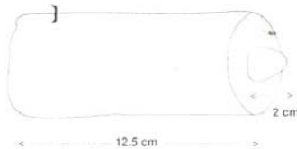
Figure 2. Simple sowing device for securing the direct sowing of Leucaena leucocephala and Gliricidia sepium alley rows at the right depth (2 cm) and the right within-row spacing (12.5 cm, or 8 plants per m alley).
